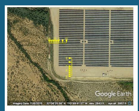
Locations of additional measures of air temperature are marked with yellow triangles. Stations were placed inside the array at 20m and 40m in from the edge of the array, at the edge of the array (0m), and outside the array at 10, 20, 30, 40, and 50m out from the edge of the array to quantify the spatial extent of the PVHI effect.
